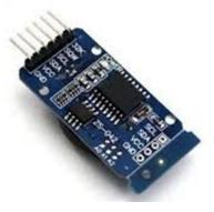
A highly accurate real-time clock module that maintains timekeeping even during power loss, used for scheduling feeding times
