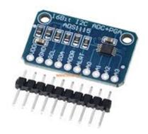
Required for interfacing analog sensors (such as the pH sensor and turbidity sensor) with the Raspberry Pi, which supports only digital inputs. The ADS1115 is a high-resolution 16-bit ADC that communicates via I<sup>2</sup>C, offering excellent precision for measuring low-voltage signals. It supports four single-ended or two differential input channels, making it suitable for connecting multiple analog sensors.
