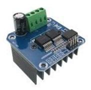
A high-current motor driver module for controlling Peltier modules with PWM signals, enabling bidirectional control and high power handling.
